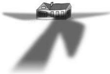
*Shadow flicker is caused by blades passing in front of the sun. Ice, debris, or anything breaking off the wind turbine blades, including the blades themselves, can impact a point 1700' from the turbine base.*
